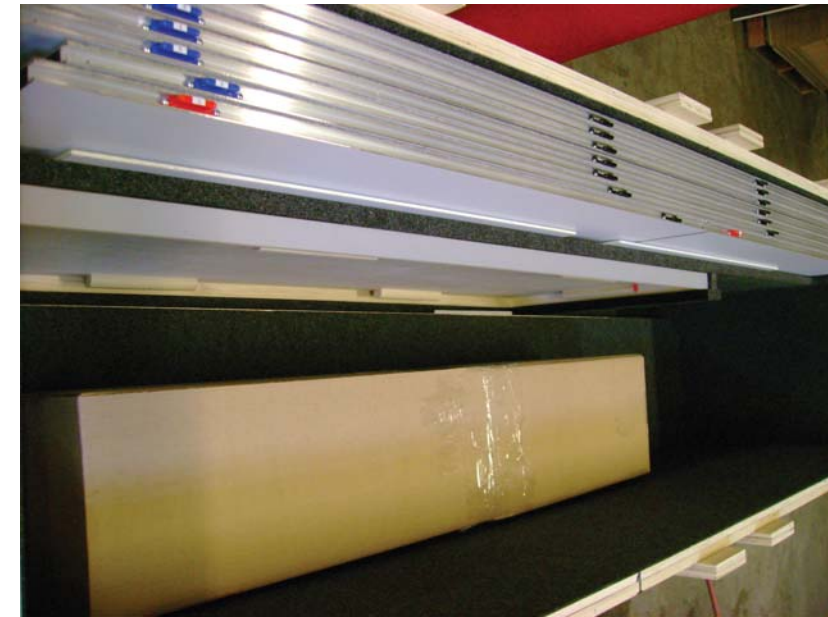
2nd Level - Contains Shelf that sits atop metal extrusions to support Tension Fabric Frame Boxes.
