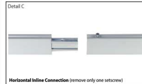
Horizontal Inline Connection (remove only one setscrew)
