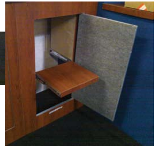
Counter with internal sliding shelf folds in as shown for packing.
