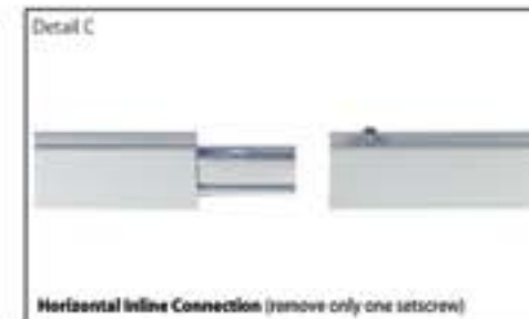
Horizontal In-line Connection (remove only one setscrew)
