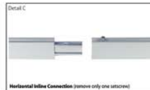
Horizontal Inline Connection (remove only one setscrew)
