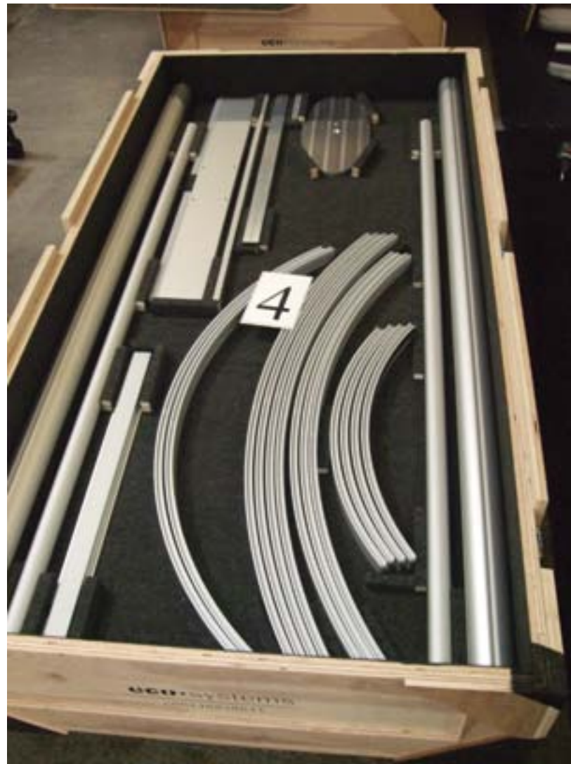
Level 4 Verticals [3,2,7,6] Monitor Mount Extrusion [17] Horizontal Header Extrusion [16] Counter Top Supports Vertical Header Extrusion [16a] Base Plates (2x) Vertical Counter Extrusion [12] Horizontal Counter Extrusions [11,11] Curved Horizontals [9a,9b,9a,9b,10,10,10,8a,8b,8a,8b]
