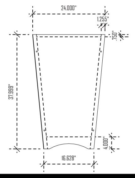
Internal dotted lines represent approximate inside dimensensions of side panels, floor, and counter edge.
