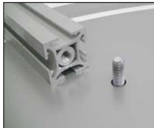
**Detail D:** Attach vertical extrusions to base plates with supplied bolts inserted through the hole in the plate. Be careful not to strip the thread.
