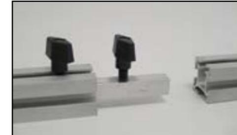
Detail E: A square connection bar with plastic T Knobs is inserted between two vertical extrusions joined end-to-end. Turn the knobs clockwise to tighten. Do Not Overtighten.
