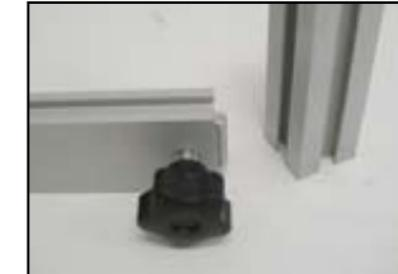
Detail F: Plastic Star Knobs are used to tighten locks where horizontal extrusions connect with vertical extrusions. Turn the knobs clockwise to tighten. Turn counter-clockwise to loosen, but do not remove knob. Do Not Overtighten.
