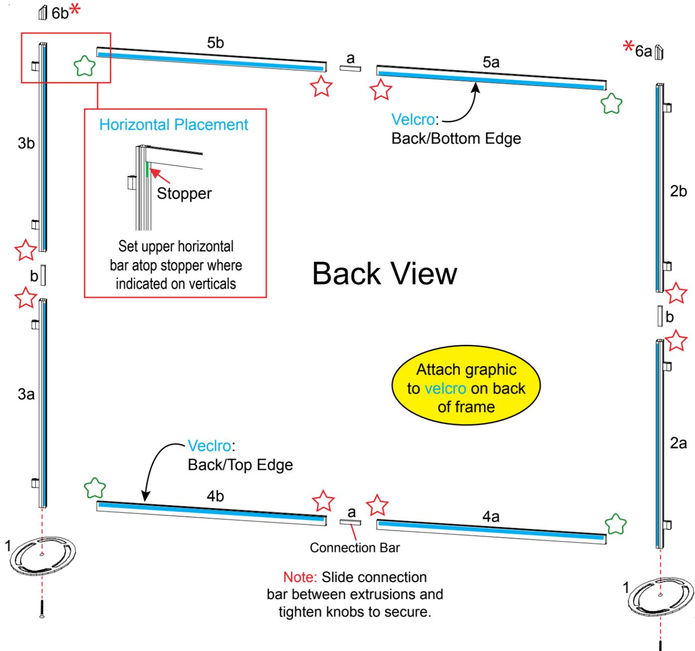
Note: Slide connection bar between extrusions and tighten knobs to secure.
