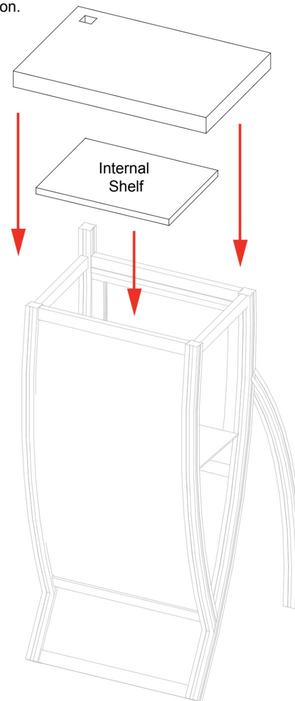
**WHEN DISASSEMBLING ALUMINUM EXTRUSION, TIGHTEN ALL SETSCREWS AND LOCKS TO PREVENT LOSS DURING SHIPPING**
